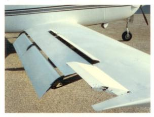
**True Fowler Flaps** Span 9/10ths of wings trailing edge. This permits a small high speed wing in the cruise regime and provides a large wing area for short take-off and landing requirements. Flaps are worm-screw driven and mechanically synchronized.
