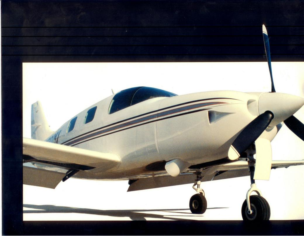
**Engine** 360 horsepower Lycoming IO540 variant. It is turbo charged, intercooled and has pressurized magnetos. The IO540 is a time-tested and proven power plant. In the 301 @ 75% power it will deliver a cruise of 270 mph and a top speed of 301 mph at 25,000 feet.
