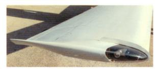
**Roll Control** Spoilers in the wing, augmented by short-span ailerons provide excellent roll authority and superior low-speed control responsiveness.
